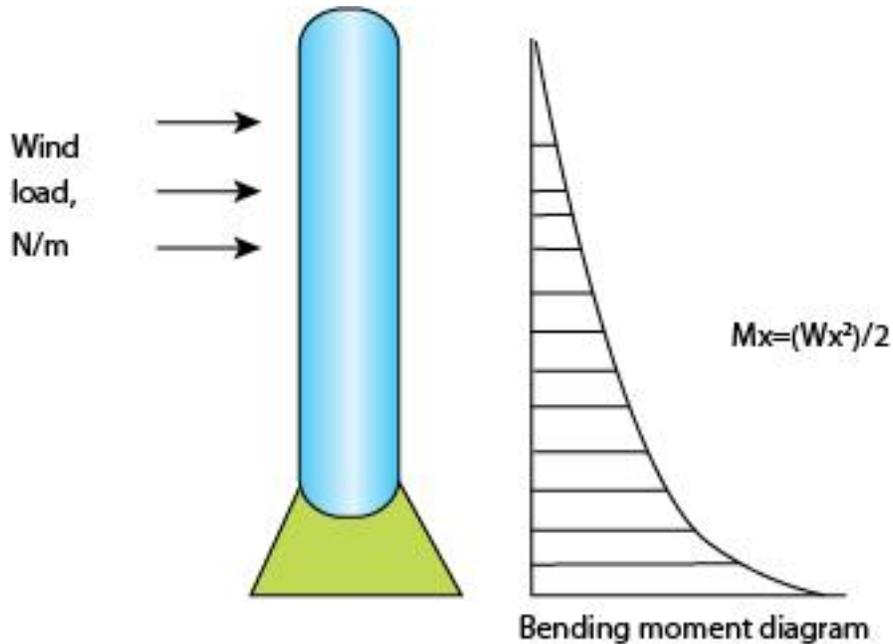
Figure 6.1: Bending moment diagram under wind load
