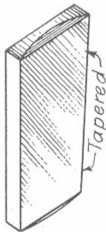
4.2.1.1F- A typical cotter with a taper on one side only (Ref.[6]).
