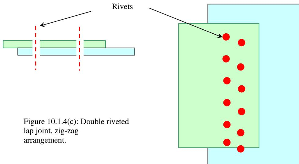
Figure 10.1.4(c): Double riveted lap joint, zig-zag arrangement.
