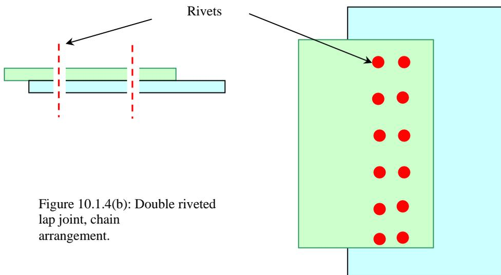
Figure 10.1.4(b): Double riveted lap joint, chain arrangement.
