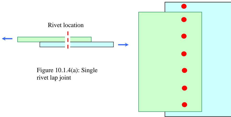
Figure 10.1.4(a): Single rivet lap joint
