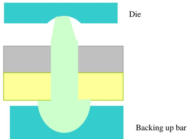
**Figure 10.1.2: Riveting operation**
