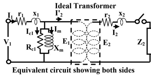
Figure 24.8: Equivalent circuit of a practical transformer.
