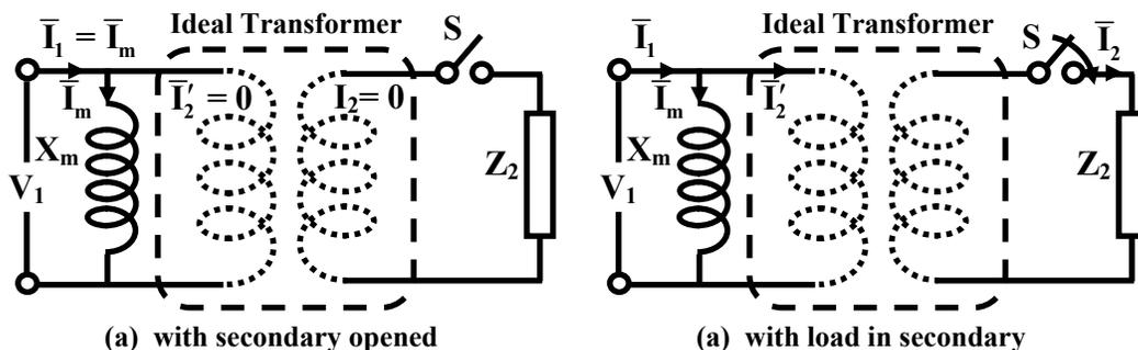
**Figure 24.3: Magnetising reactance to take  $I_m$  into account.**
