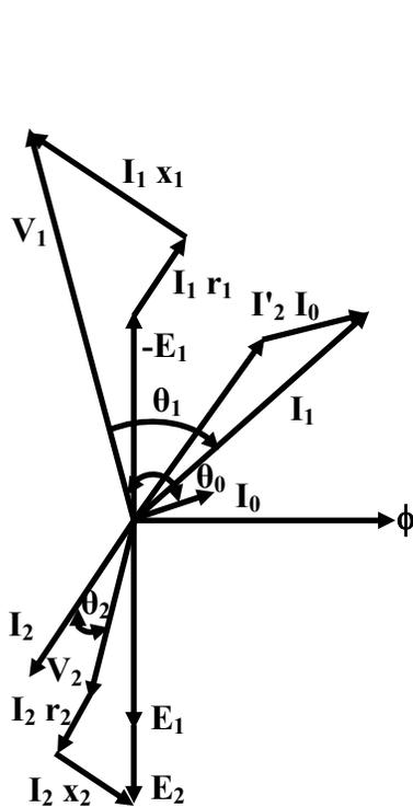
**Figure 24.10: Phasor diagram of the transformer supplying lagging power factor load.**
