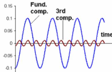
**Fig. 34.2(e): Normalized fundamental and 3<sup>rd</sup> harmonic components of load current for  $L/R = 2T$**
